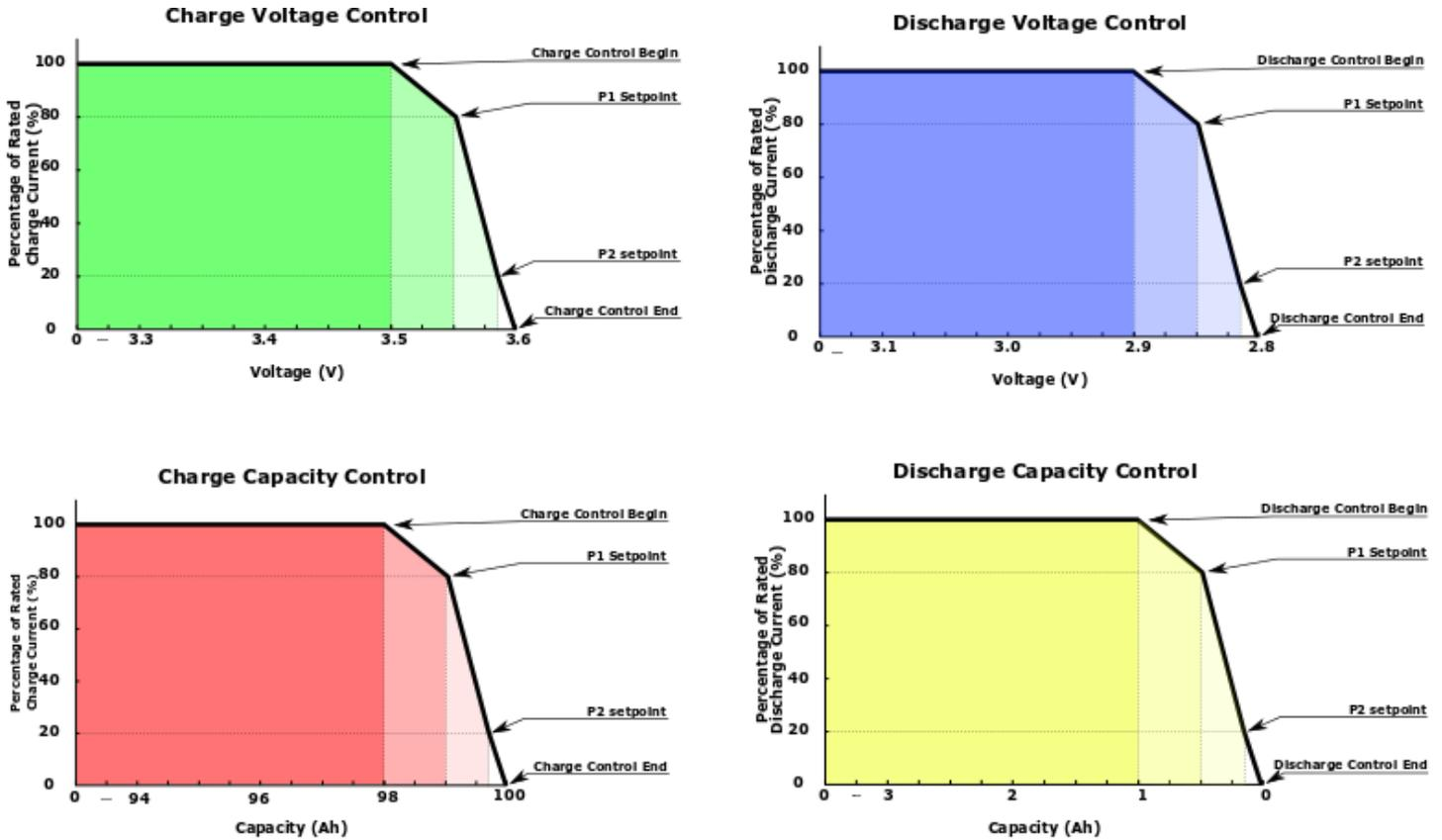
Figure 9: Voltage and capacity based charge and discharge control
