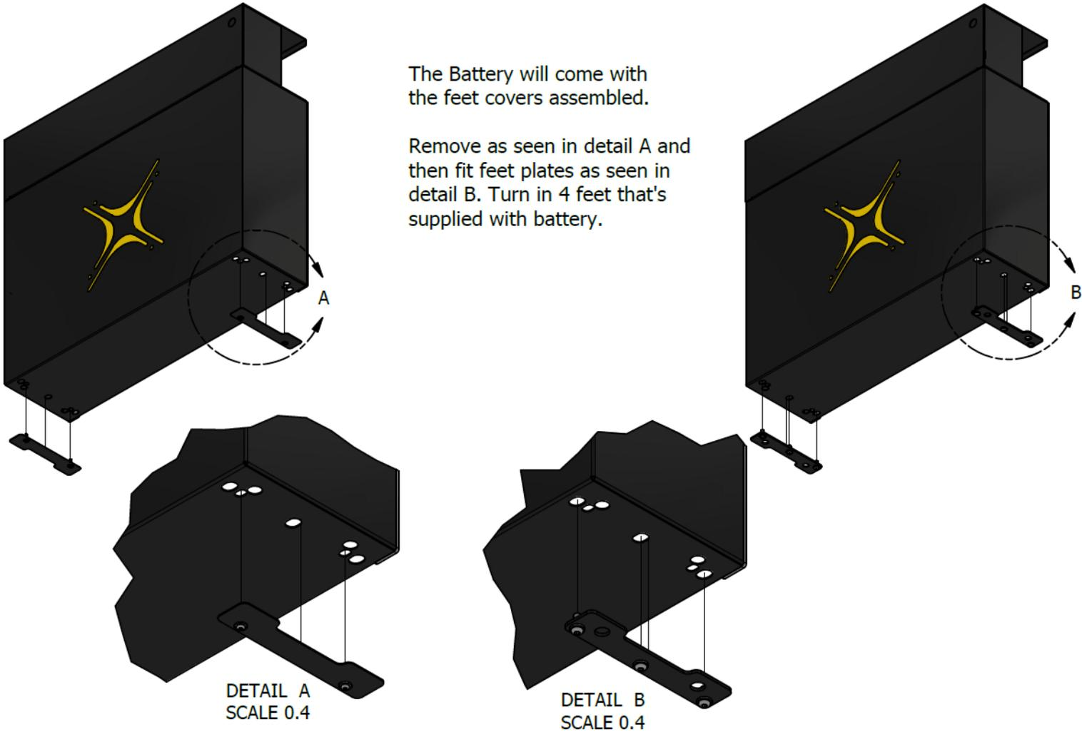
Figure 3c: Battery feet - installation of battery feet
