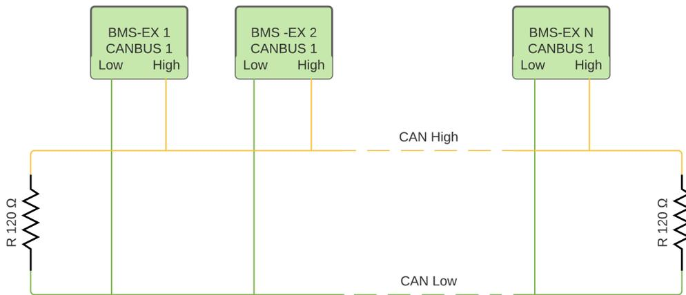
Figure 10: BMS communication ports
