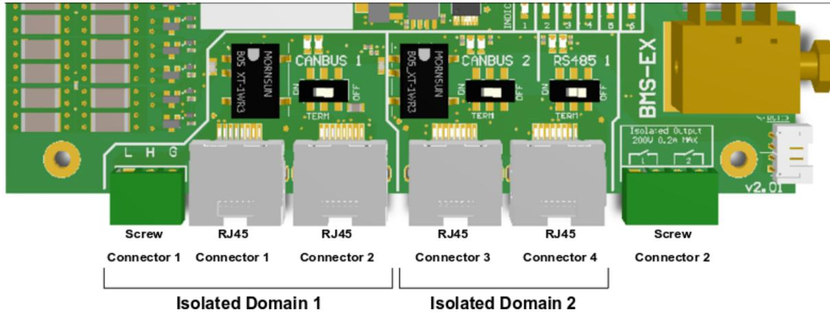
Figure 8: BMS communication ports
