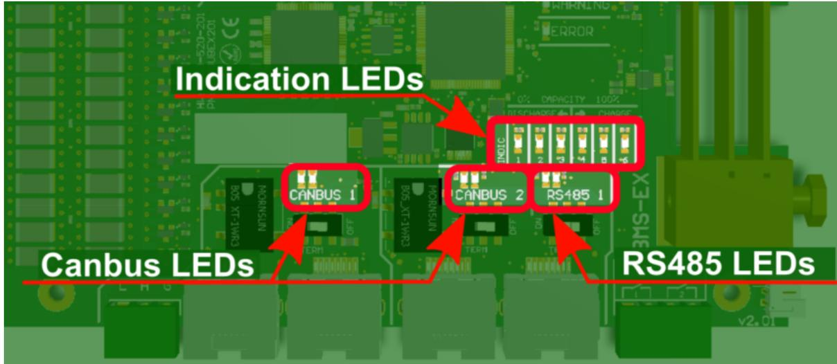
Figure 7: LEDs on the BMS
