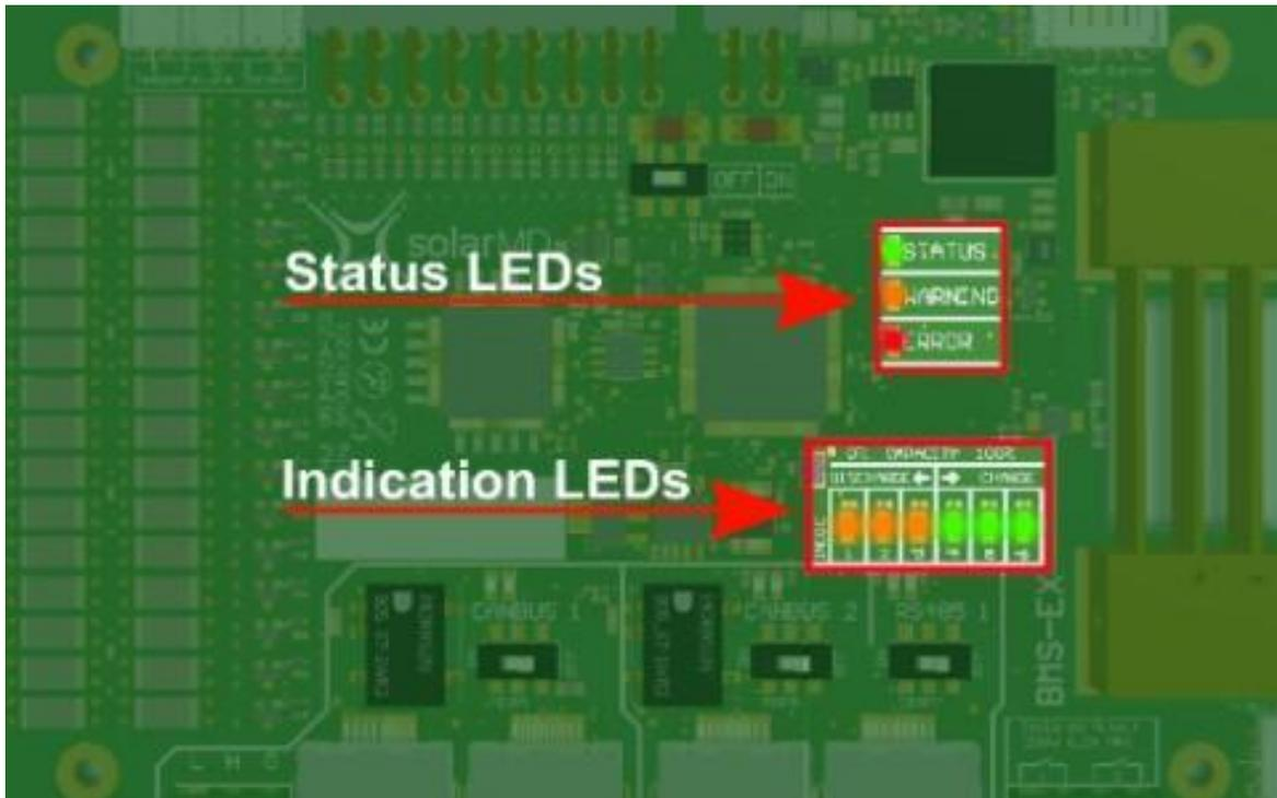
Figure 11 : Display general warnings and errors, main status LEDs and indication LEDs.
